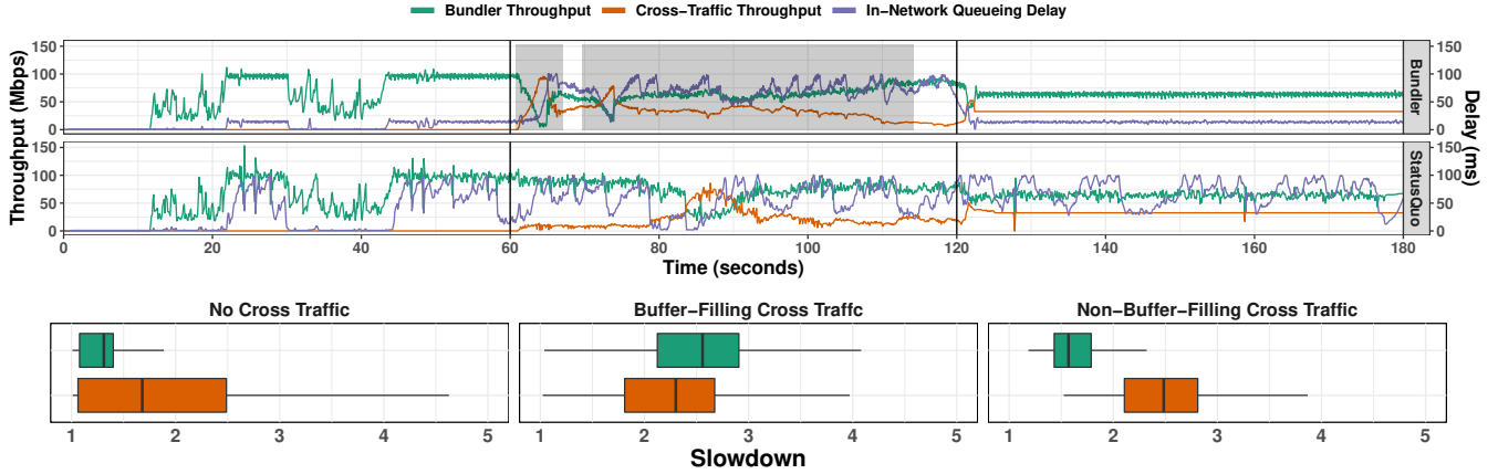
Figure 10: Bundler’s scheduling ability depends on the characteristics of the cross traffic over time. In this experiment, there are 3 periods: from 0 to 60 sec., there is no competing traffic, from 60 to 120 sec. there is buffer-filling cross traffic, and from 120 to 180 sec. there is non-buffer-filling cross traffic. The box-plots below each period show the distribution of short flow FCTs during that time. During the period with buffer-filling cross traffic, Bundler detects its presence and competes fairly. The shaded region indicates time Bundler spent in buffer-filling cross-traffic mode (§5.1).
