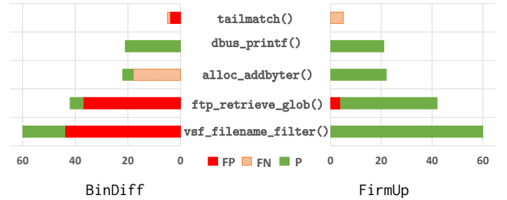
Figure 6. Labeled experiment comparing BinDiff with FirmUp, showing that BinDiff encountered over 69.3% false results overall compared with 6% for FirmUp
