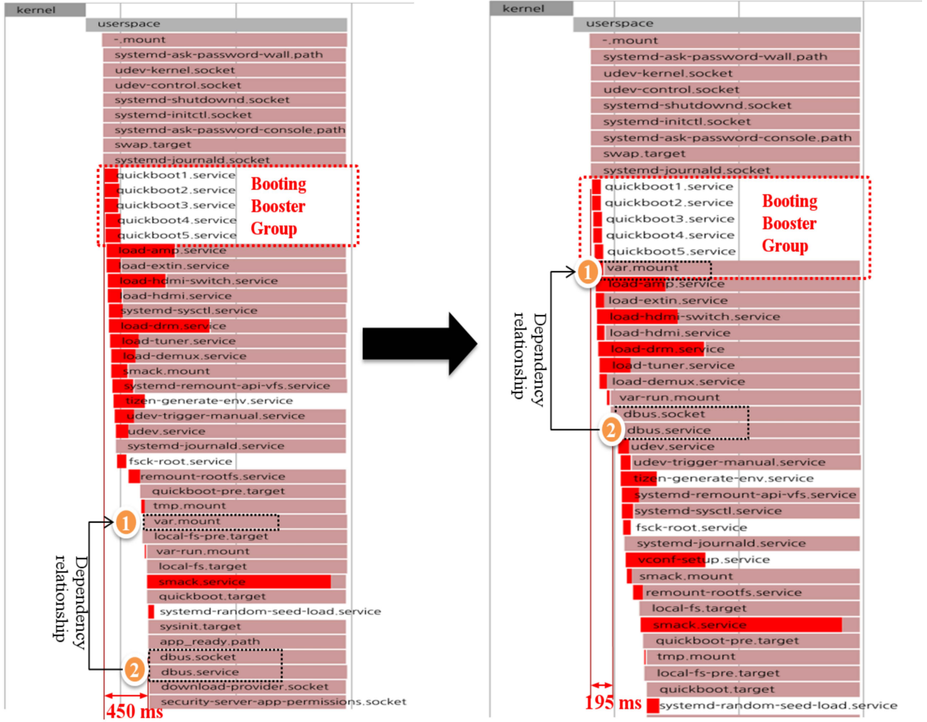
Figure 7. Graphs of systemd-bootchart showing the effects of BB Group by adding var.mount into BB Group to advance the launching time of dbus.service
